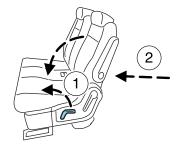
After entering the 3rd row, pull back the seatback until it latches. This will latch and lock the seatback and the seat track. The seatback and seat will not return to their original position.
